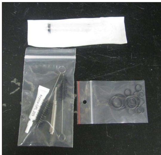
FIGURE 6.3 - YSI 6-SERIES SONDE MAINTENANCE KIT: O-RINGS, O-RING LUBRICANT, CLEANING BRUSHES, PROBE INSTALLATION TOOL, SYRINGE FOR SENSOR PORT CLEANING.
