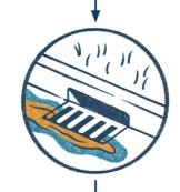
Stormwater enters storm drains on roads and flows through underground channels
