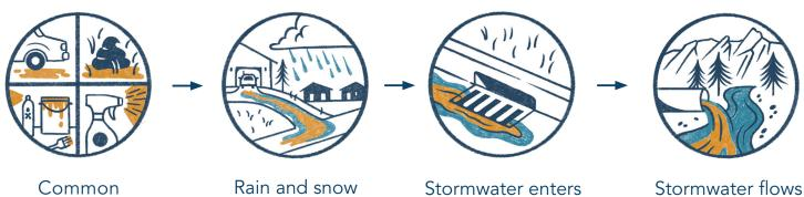
Common household activities can be sources of pollutants pick up pollutants and carry them into roads as stormwater stormwater enters storm drains on roads and flows through underground channels Stormwater flows through these channels directly into local creeks without being treated
